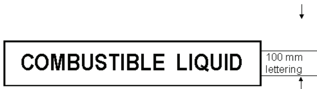
Figure 5—Placard for C1 combustible liquids
